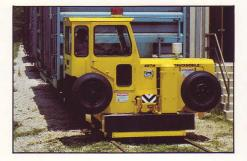
This single coupler vehicle is a real workhorse capable of moving seventeen 100 ton cars.
