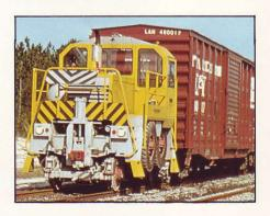
Capable of moving fifty 100 ton cars and a 30 MPH rail speed, the 11TM is built for speed and power for long hauls as well as spotting and switching operations.
